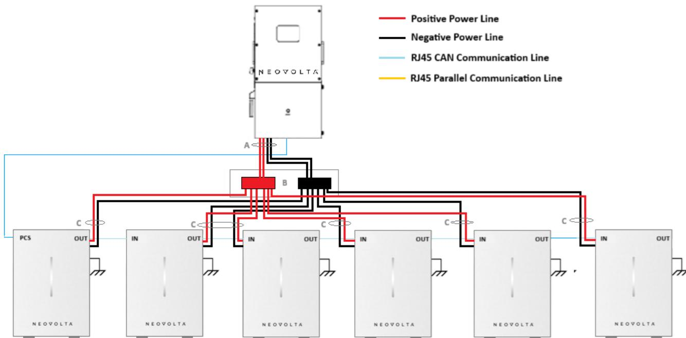
**Note:** To ensure balanced power distribution and optimal system performance, verify that all inverter-to-DC bus cables are of equal length, and likewise, all battery-to-DC bus cables are matched in length.
