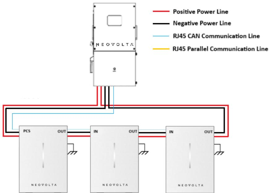
**Note:** To ensure balanced power distribution and optimal system performance, verify that all inverter-to-DC bus cables are of equal length, and likewise, all battery-to-DC bus cables are matched in length.
