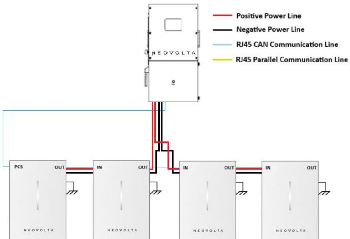
**Note:** To ensure balanced power distribution and optimal system performance, verify that all inverter-to-DC bus cables are of equal length, and likewise, all battery-to-DC bus cables are matched in length.
