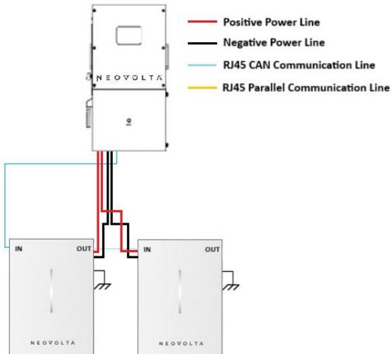
**Note:** To ensure balanced power distribution and optimal system performance, verify that all inverter-to-DC bus cables are of equal length, and likewise, all battery-to-DC bus cables are matched in length.
