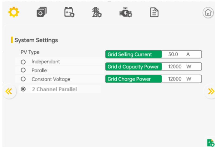
When enabled, the inverter treats MPPT 1 & 2 as a combined single MPPT, and MPPTs 3 & 4 as a second combined single MPPT.
