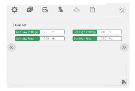
The generator's input voltage and frequency are monitored and controlled according to the protection settings on this page.
